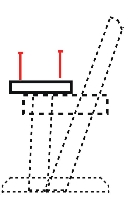
Place the back flush to the top and centered with the bottom plank, and screw in using 3 screws on each side.
